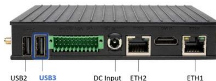
Figure 2: Horizon Power's SGD hardware and port overview 1
