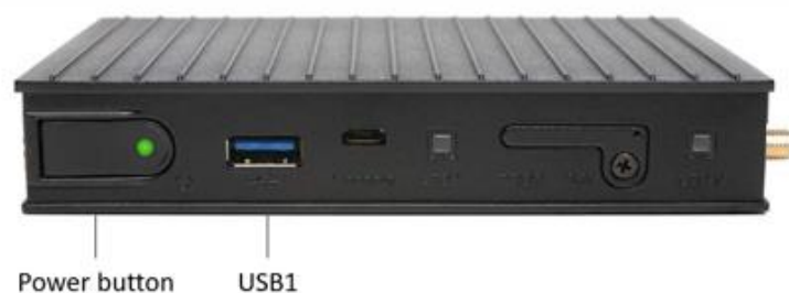
Figure 3: Horizon Power's SGD hardware and port overview 2
